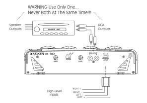
The use of twisted pair interconnects is recommended for all installations to minimize noise. When routing these cables through the automobile, try to keep them away from factory wiring harnesses and other power wiring. If you need to cross any of this wiring do so at a 90 degree angle to reduce the potential of alternator noise and electrical interference.
